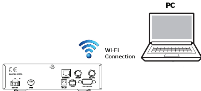
Figure 27 : ACU to PC Wifi Connection
